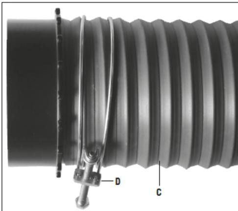
4. Attach the other end of the suction hose using a hose clamp and hose coupling.
